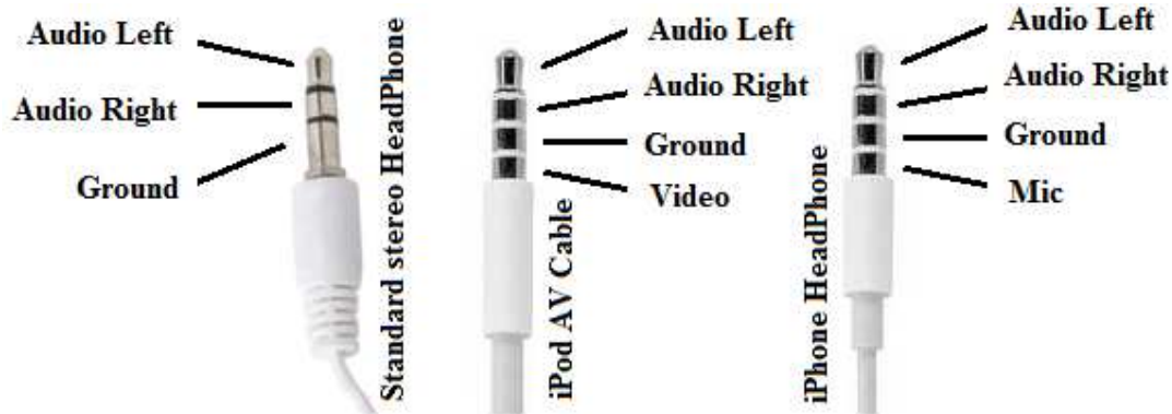
Figure 1.3: Comparison of different Headphone plugs
