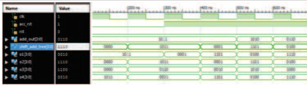
Fig. 3 Simulation Results of The shift Accumulator.
