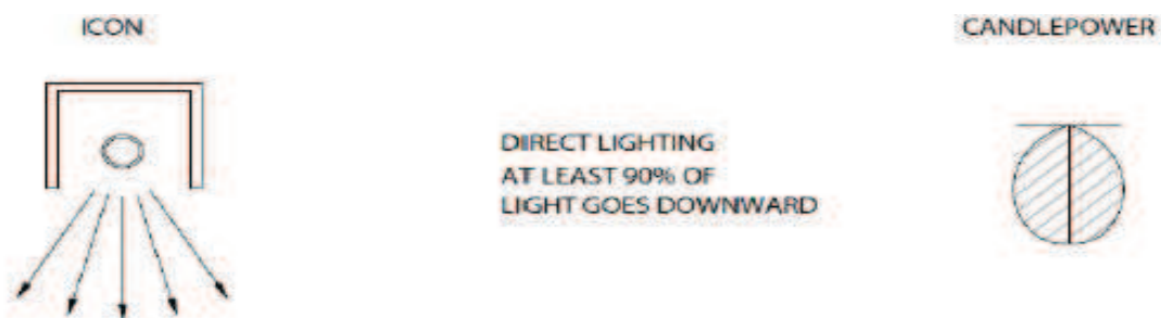
Fig. 1: Direct (90 to 100 percent of the Light is Directed Downward for Maximum Use.
