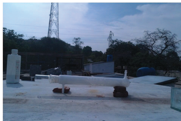
Fig 6: experimental setup of tubular design with TiO 2 coating
